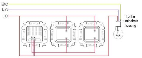
2.5 Dimmer with LED Strip (Single-Color or White-Emitting) This setup enables lighting control from multiple locations.
